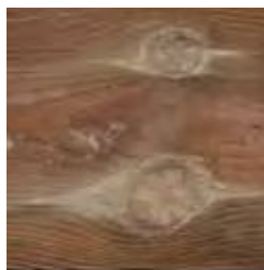
Round knots/Nodos redondos/ Noeuds ronds/Runde knoten / Nodi rotondi/ Ronde kwasten/ Nós redondos
